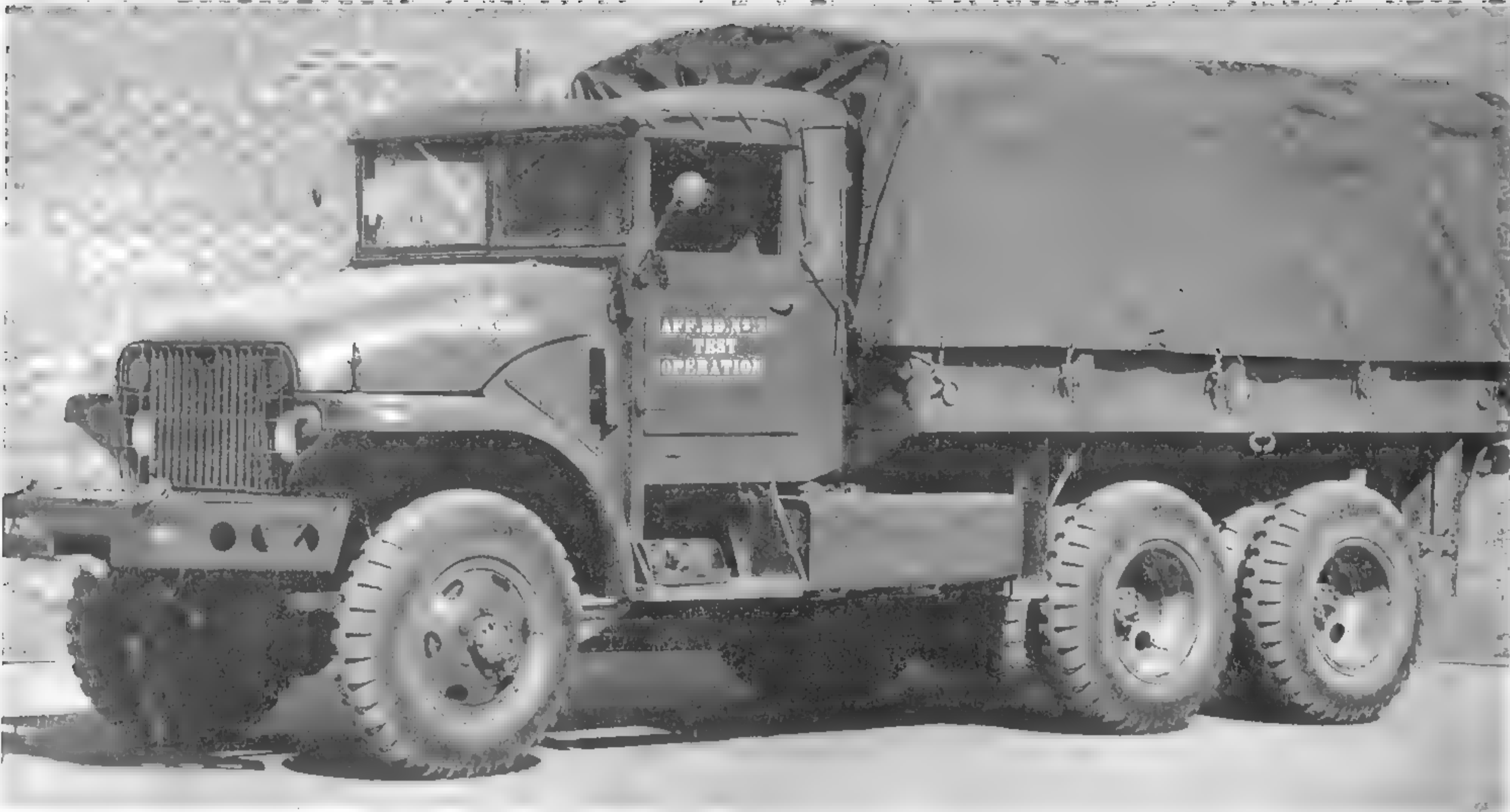
The dual-wheel equipped XM211 cargo truck was also demonstrated to the Army Field Forces Board Number Two. Two different-size fuel tanks, differing in length and depth, were used on the G-749 series trucks. The tank shown here is the typical one. Mass production of the dual-wheel version of this truck began before it was officially standardized, resulting in an abundance of XM211 trucks being built. (Photo courtesy of the Patton Museum)
